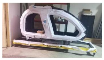
ii. Bucks – are used to produce additional molds
