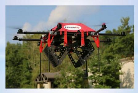
Designed to fly and be charged from a Workhorse electric truck, HorseFly is powered by 18650 lithium ion cells, can carry a 10 lb. package 20 miles in almost any weather.
